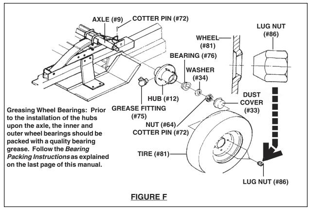
Place a Wheel/Tire Assembly (part #81) onto each Hub (part #12). Secure each Wheel/Tire assembly firmly to the Hubs, using the Lug Nuts (part #86)
